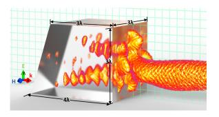
The incident field is a plane wave of 625 nm, and the cuboid has refractive index of 1.46.
