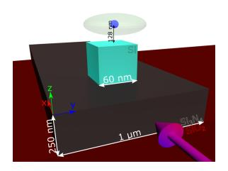
For an incident field of 2400 nm, adding a subwavelength Silicon cube changes the field on top of the waveguide.
