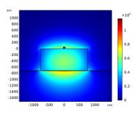
For an incident field of 2400 nm, adding a subwavelength Silicon cube changes the field on top of the waveguide.
